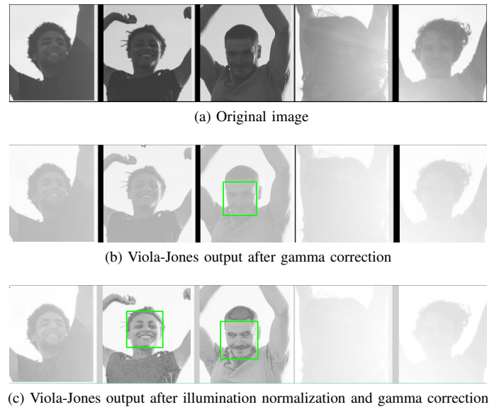
Fig. 1: Impact of illumination on face detection.
